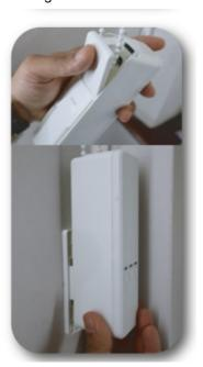
6. To change your motor direction, press & hold the "UP" button for 6 seconds until the LED flashes to confirm.
