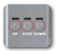
2. To restore to factory settings, press & hold the UP and DOWN arrow for 5-8 sec. until the LED flashes. To release the motor off the bracket, push the button underneath the motor
