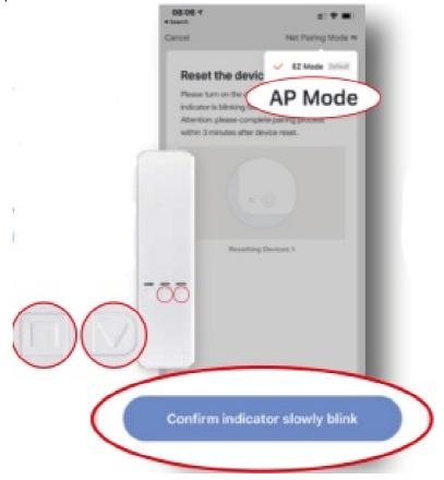
Press and hold the "up" and "stop" button for 6 seconds on the motor until the LED flashes
