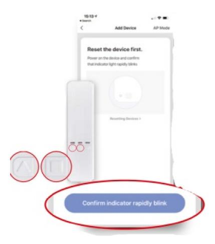
Press and hold the "up" and "stop" button for 6 seconds on the motor until the LED flashes
