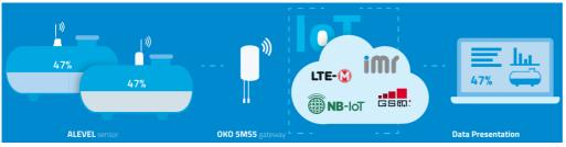
OKO 5MS5 can be conveniently located close to the tank, on well-maintained, gas or ventilation pipe line, at a height ensuring the best possible network coverage. OneOKO 5MS can retransmit level signals from up to 6 smart level sensors. OKO 5MS5 can interface any Lot or serial device to the Cloud. Its flexible, extendable design allows it to be used in different configurations.
