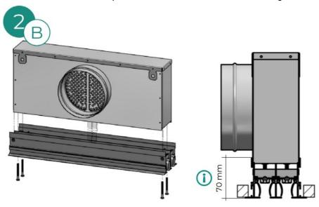
**Note:** Don't forget to regulate the airflow via the butterfly damper.
