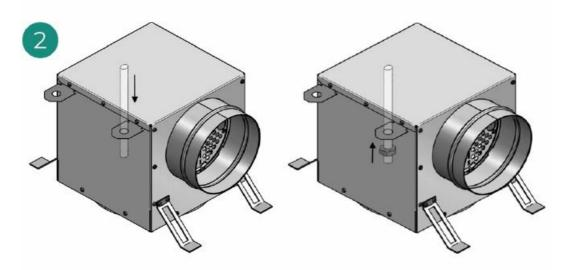
3. Fix the diffuser to the plenum using the screw provided.
