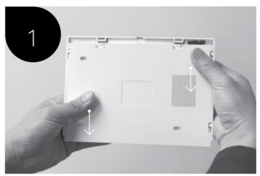
Push out, and remove the indicator sticker from the mounting plate to expose the hole of the RJ12 socket.
