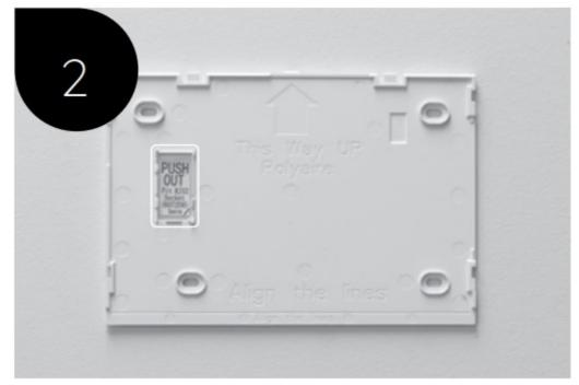
Place the mounting plate in an appropriate position on the wall (about 1.5m above the ground, away from direct sunlight) and make a suitable size hole in the indicated label position for installing the RJ12 **connector.**
