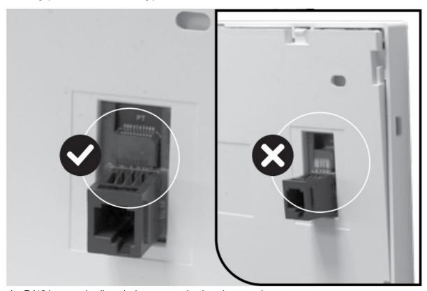
Ensure the RJ12 is properly aligned when connecting it to the console.
