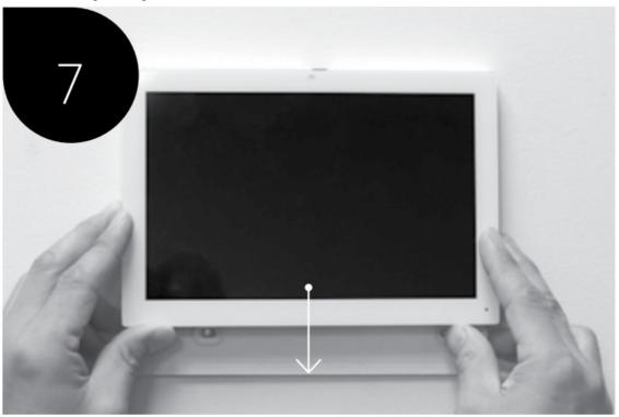
Align and slide on the console to complete the installation.
