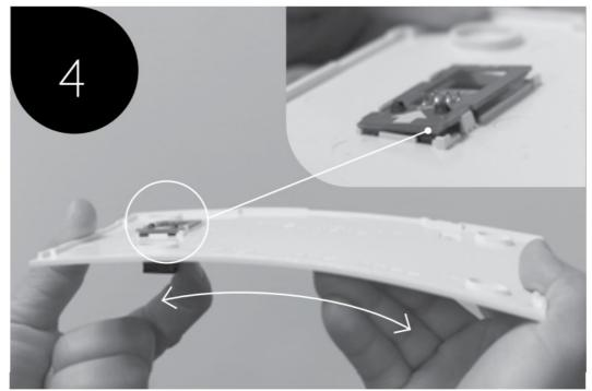
Align the left side of the RJ12 against the two clips, push back slightly to allow the right side of the RJ12 to slide underneath.
