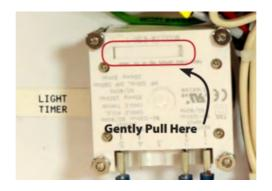
**Step 1:** On the back of the timer use a small flathead screwdriver or similar to pull the battery compartment from the timer.
