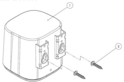
recommend measuring the distance between the two large mounting points and drilling two M4 screws into the
