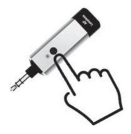
Single press the button to turn on the device, the LED indicator will be flashing blue and red ( ready to be paired ).
