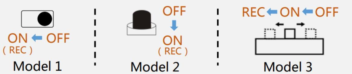
The diagram illustrates three models of the device and their recording switch positions. Model 1 has a toggle switch with 'ON (REC)' and 'OFF' positions. Model 2 has a rotary switch with 'OFF' and 'ON (REC)' positions. Model 3 has a rotary switch with 'REC', 'ON', and 'OFF' positions. Dashed vertical lines separate the three models.
