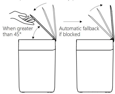
3.6 If the flip lid is in normally open mode, tap the touch key once, or close the flip lid directly by hand, it will exit the normally open mode.
