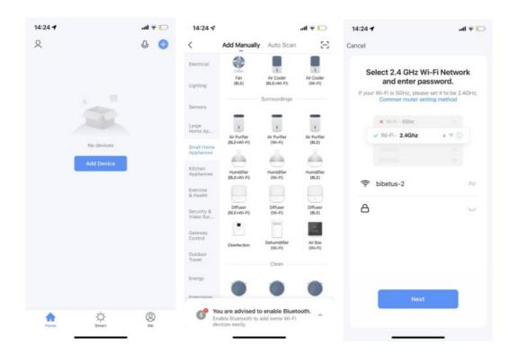
4. In order to add a device to the application, it must be running in WiFi connection mode, which is indicated by a flashing WiFi icon on the device display. If the WiFi icon does not flash, turn off the device and hold down the MODE button for seconds. Repeat until the icon flashes quickly. Then check the message box "Confirm that the light is flashing fast" in the application and go to the next step
