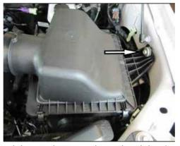
5. Remove the 8mm fender bolt in the air box and remove the entire air box/scoop assembly from the vehicle.
