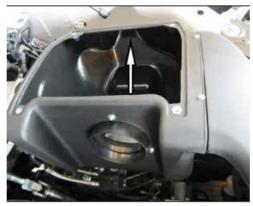
12. Secure the Airaid Air Box to the inner fender using the 8mm bolt removed in step 5.
