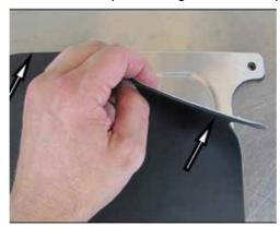
20. Remove the protective film from the top of the Air Box Lid. Prepare the underside for the Lid Gasket by cleaning it using a prep-sol or equivalent. Carefully apply the self-adhesive Gasket onto the Lid as shown.
