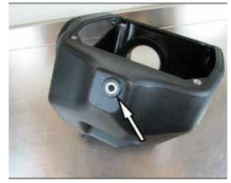
7. Insert the 5/8" Grommet and Spacer into the opposite side of the Airaid Air Box.
