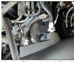
18. Reconnect the breather lines to the Aluminum Fittings in the Intake Tube. When properly installed a distinct "
