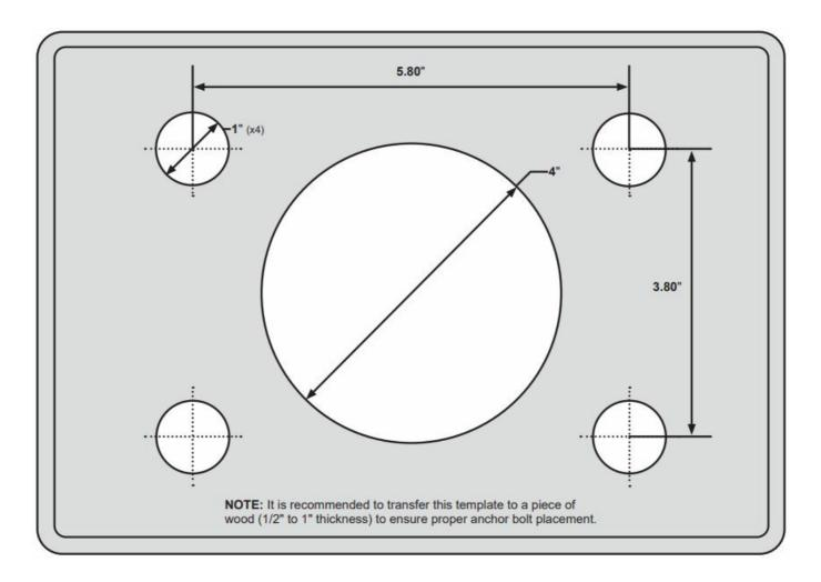
**NOTE:** It is recommended to transfer this template to a piece of wood (1/2" to 1" thickness) to ensure proper anchor bolt placement
