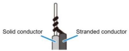
2. Bend the tip and solder it. Make sure no lead wire sticks out.
