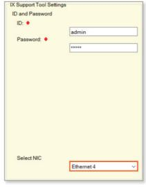
This menu cannot be accessed from the Programming Wizard. If this is the first installation in the IX Support Tool, create a placeholder system, associate nothing, and click Next or Finish on each window until the Edit drop-down is available.
