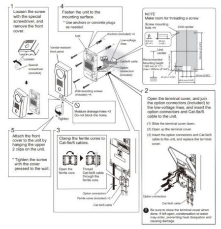
• IX-DVF, IX-DVF-P, IX-DVF-2RA, IX-DVF-RA, IX-DVF-L, IX-SSA, IX-SSA-2RA, IX-SSA-RA (flush mount)
