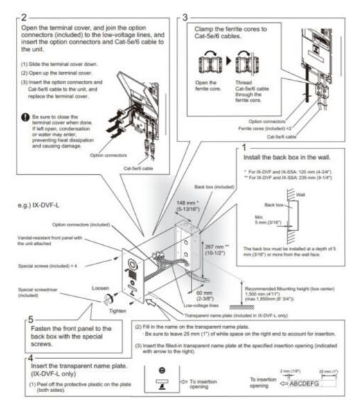
Camera View Area and Mounting Location (IX-DV, IX-DVF, IX-DVF-P, IX-DVF-2RA, IX-DVF-RA, IX-DVF-L)
