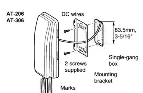
Mount the intercom on bracket, aligning at the marks. Pull down on bracket, until it properly locks. Terminal section is on the back side. Do not disassemble the unit. For surface wall cable run, outlet hole is provided on the top or bottom of chassis.
