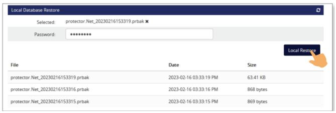
The AC-HOST can also be restored from backups located on the PC accessing its web interface, or from elsewhere on the local network. Enter the System Manager password created before. Click Browse to locate the database, then click Restore.
