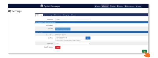
During initial setup, make sure that the AC-HOST has a network connection, and that either NTP is set to NTP Enabled, or click Sync Time from Internet. This is required to successfully apply the AC Nio license. Once the license has been applied, a manual time can be used instead.
