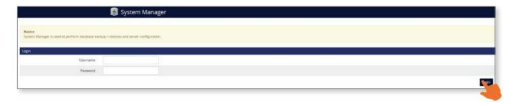
This will open up a home screen that provides options to restart or shut down features of the AC-HOST, as well as the device itself. It is a good idea to change the password from the default at this time. Enter the acaccess password, then enter in the new on on the New Password and Confirm Password lines. Record the password in a known location, then click Change.
