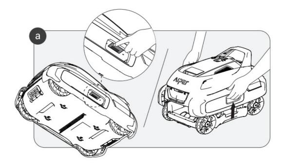
b. Lift and set aside the upper shell, then remove the filter to begin cleaning.
