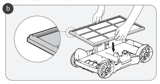
c. Align the upper shell with the chassis and press down slightly to buckle the parts together.
