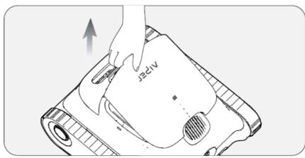
• b. Remove the filter basket by lifting its handle.
