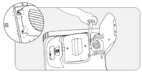
• b. Remove the screws and drain the cover.
