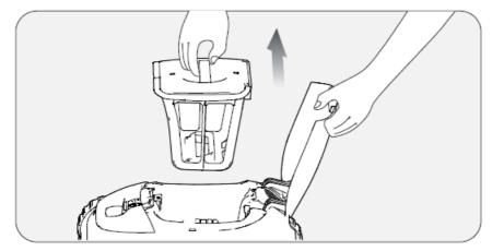
• c. Press the top shell latch of the filter basket and at the same time pull up on the top cover handle to open the filter basket.
