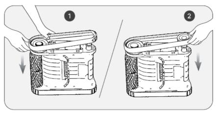
• e. Re-install the white guide sleeves by aligning their D-shaped openings with those of the shaft sleeves.
