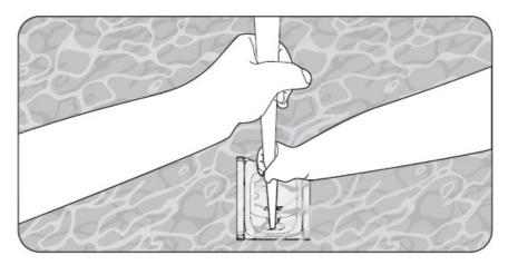
• g. Hold the handle and allow the device to drain any stored water.
