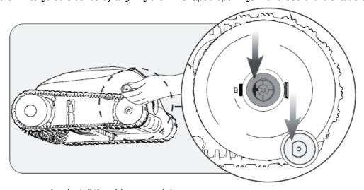
• f. Tighten the screws and re-install the side cover plate.
