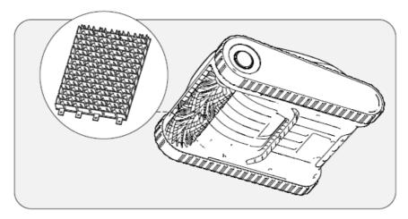
• b. After all the silicone buckles are pulled out, replace the roller brush belt with a new one. Align the silicone buckles with the fixed slot and pull them outward. They can be fixed after passing through the slot.
