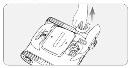
• c. Remove any objects entangled in the drain fan blades, and then re-install the drain cover and screws.
