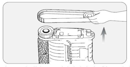
• d. Align the gears on the new tracks with the gears on both wheels, then install the rear wheels and tracks together back onto the shaft sleeves.
