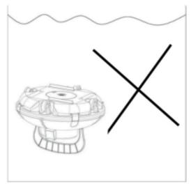
b. Install the swing plate and floating handle before using.
