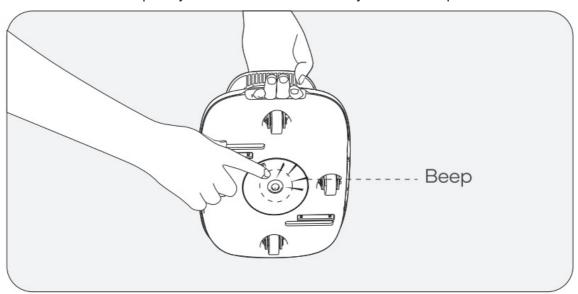
4.3 If your device has powered off due to low battery against the edge of your pool, the device will beep intermittently for two minutes.
