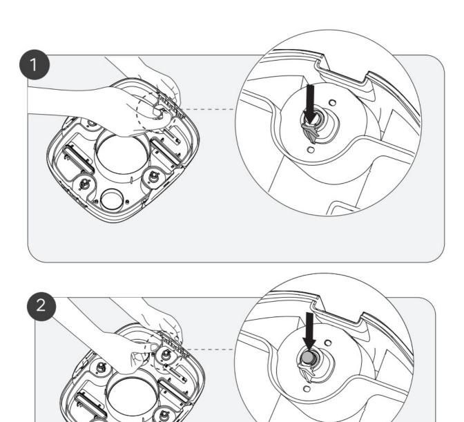
3. Insert the new wheel stem by first aligning it with the two small holes of the wheel socket. You should hear a clicking sound when the wheel has locked in place.
