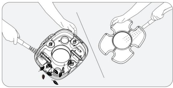
4.8 Put the filter back into your device. Return the Top Shell to the device. You will hear a click when Top Shell is securely attached to your device.
