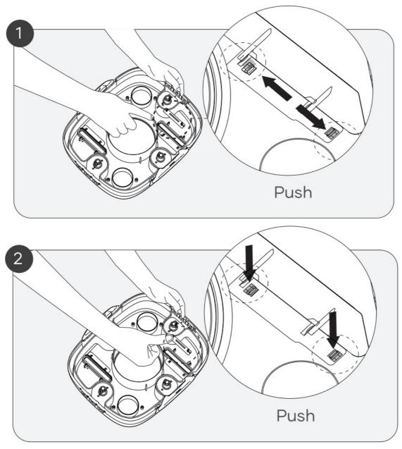
Press the locking pins down to release the brush.
