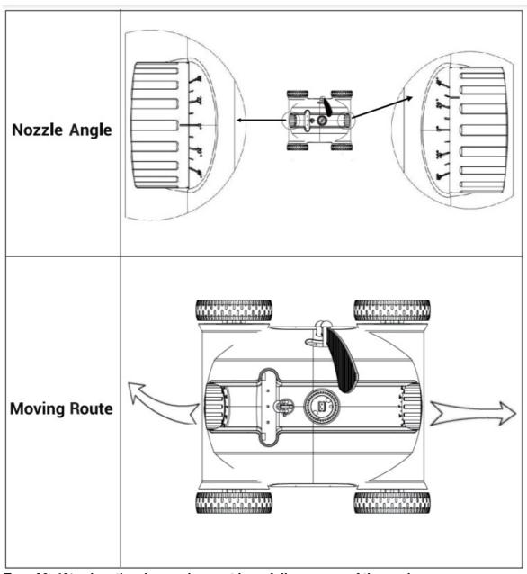
Setting Two: 00–40°, when the cleaner does not have full coverage of the pool.
