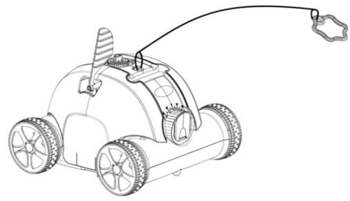
b. Install the swing plate Insert the swing plate in the place Indicated in the fig.
