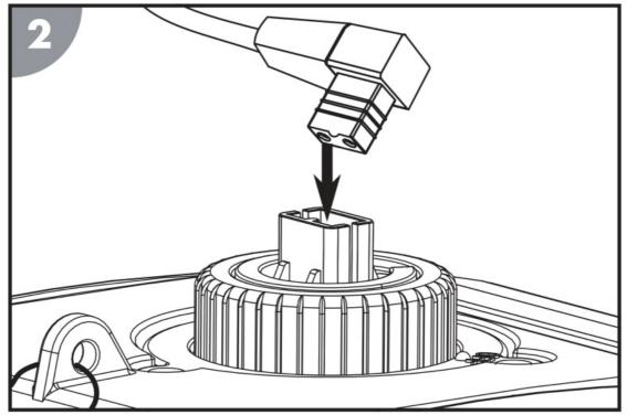
Attach the protective cap to the charging plug
