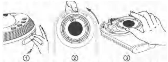
4. **Note:** It is recommended to replace the film disc in the powered-off state.
