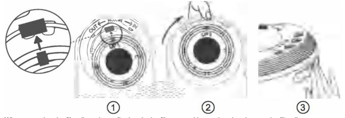
3. When removing the film disc, please firmly grip the film gear with your hand and rotate the film disc counterclockwise to align it with the groove of the film disc card slot before taking it out.
