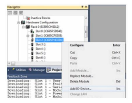
Select ABCC-PRT2P device from HMS Industrial Networks and click 'OK.' If it isn't listed you will need to import the GSD file which can be found on the controller's web interface.
