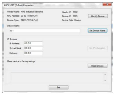
For simplicity, set the device name to 'tc-1' and hit 'Set Device Name,' then 'Exit.' The Gen 4 controller now has a device name but not an IP address.
