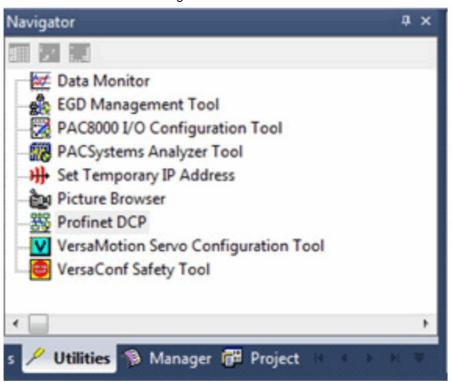
Double click 'Profinet DCP' to bring up the discovery tool. From the drop-down menu, select 'Local Area Connection and press the 'Refresh Device List' button. This should list all the Profinet devices on the network.
