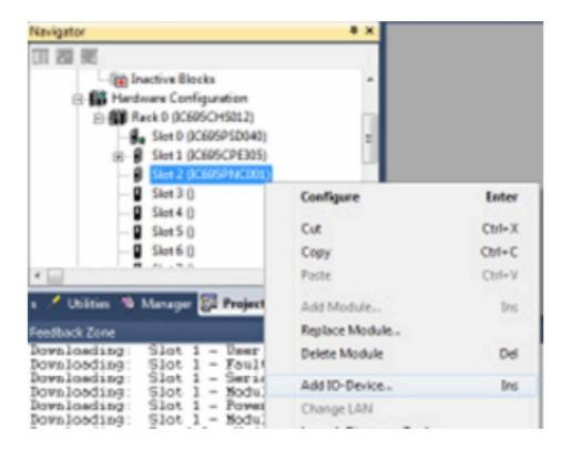
When the Catalog box appears, click on the 'Bus Controller' tab and select 'IC695PNC001 – RX3i PROFINET Controller (2 SFP)'. Click 'OK' when finished.
