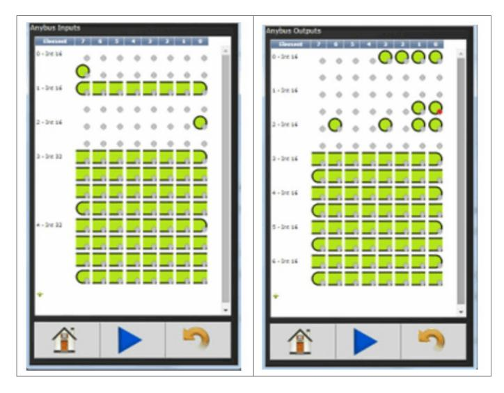
To verify that the communication is successful, navigate to the 'Default Tables' in the Proficy Machine Edition software and either look at the analog inputs coming in from the ANY BUS Outputs on the Gen 4 controller or force the analog outputs to the ANY BUS inputs. Make sure to start the PLC controller first.
