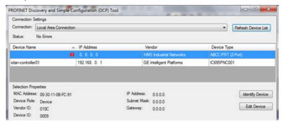
The GE PNC001 scanner card has a Device Name of 'Nolan-controller01' and is at IP address 192.168.0.1. If the Gen 4 controller has never been configured it will not have a Device Name or IP address yet. The Gen 4 controller will always show up as HMS Industrial Networks ABCC-PRT (2-Port).
