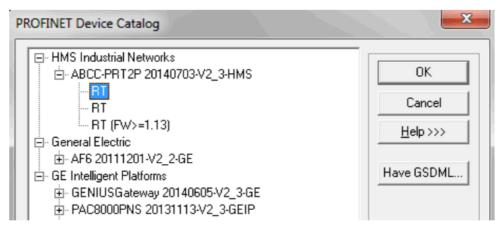
This will add a new device with the default device name of 'ABC-prt-2-port.' Edit the properties of this device and change its Device Name to tc-1 to match the controller we have on the network. This will also assign an IP address to the Device name.
