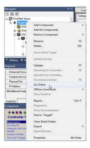
Notice that the target symbol has changed to online/monitor mode and also indicates that the current settings do not match the existing PLC settings.
