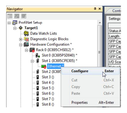
The PLC in this example has IP address 10.10.13.201 (if this is a new device, check for the default IP address value). Set the IP address to this value with subnet 255.255.255.0.
