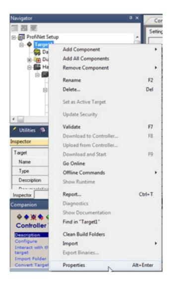
The properties of any device are shown in the 'Inspector' window. From this menu, scroll down to the bottom and enter IP address 10.10.13.201. Hit enter when finished.
