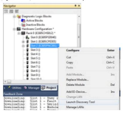
Click 'Refresh Device List and the controller (tc-1) should show up as 'Not assigned.' Right-click on the PNC001 card in the hardware configuration and select 'Add I/O Device.'
