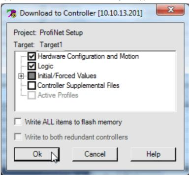
Once the process finishes, 'Target1' indicates online/programmer mode and that you have the same settings on both the PC and PLC.
