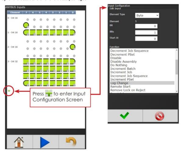
Example of the Anybus Input screen with five Inputs set up.
