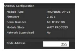
Node Address: Configures the Anybus node address for controller.
