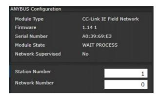
**Station Number:** Configures the station number for the controller. Valid entries are 1 - 64. **Network Number:** Configures the network number the controller is on. Valid entries are 0 - 239.
