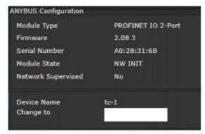
Device Name: Configures the device name of the controller.
