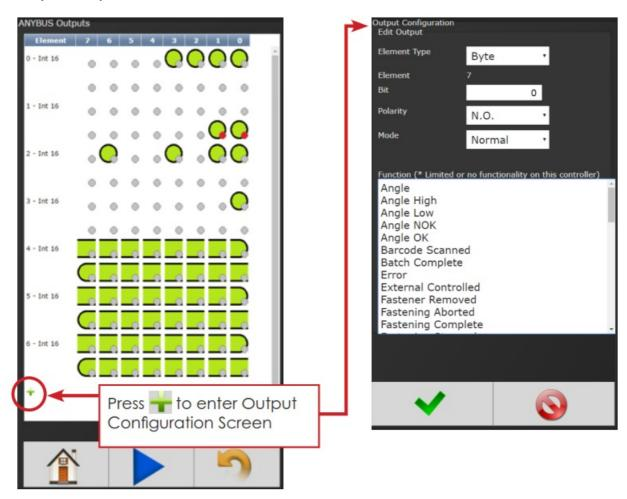
Example of the Anybus Output screen with five Outputs set up.
