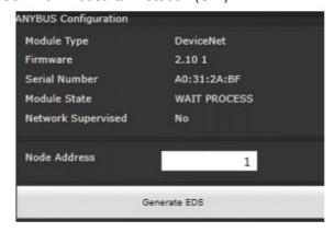
DeviceNet covers the main part of the applications where small to medium amount of data with short to medium cycle times (1ms to 500ms) can be exchanged in the network.
