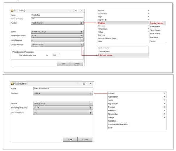
• When the configuration is finished save and transmit it to the logger (MXG 1 in the example) using the software's top left keyboard.
