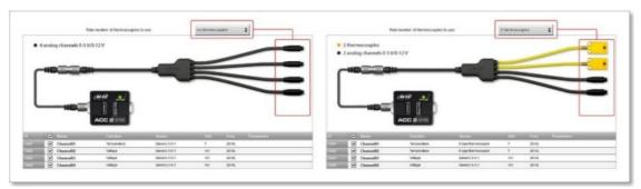
• ACC2 supports up to four K-type thermocouples. Once the number of thermocouples (s) to be connected is fixed the software warns you and the corresponding channel(s) switches to "Temperature".
