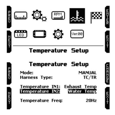
Harness Type: indicate the extension of the sensors connected to the MyChron5S, it could be:
