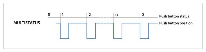
No matter the mode the pushbutton is set you can also set a time threshold: in this case, the pushbutton is set at two different values that you may define depending on how long you push it.
