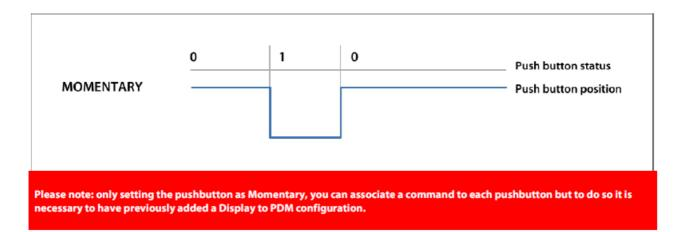
**Please note:** only setting the pushbutton as Momentary, you can associate a command to each pushbutton but to do so it is necessary to have previously added a Display to PDM configuration.
