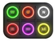
**AiM Keypad Open Version** is the new range of compact expansions based on the CAN bus. It is available in different versions according to the number of pushbuttons whose status is transmitted through the CAN bus. Both buttons and CAN messages are fully configurable through the USB connection using AiM RaceStudio 3 Software. Each button can be set as:
