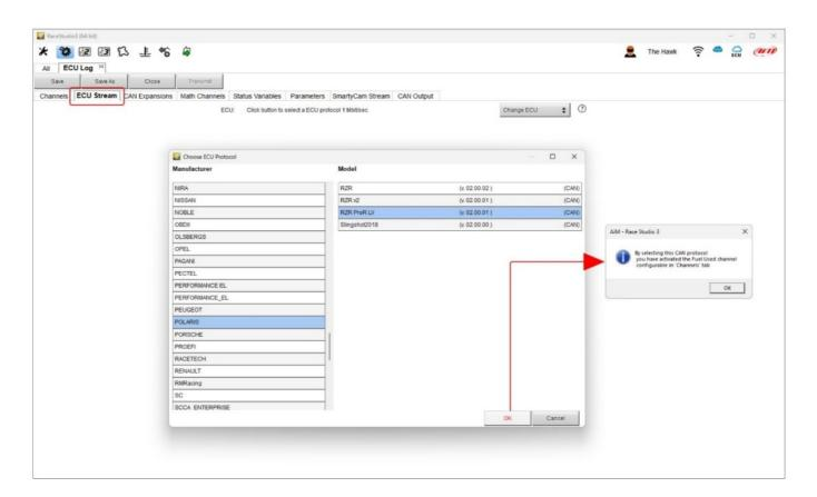
Selecting an ECU that supplies information about fuel level the software informs the user as shown above and the corresponding channel is enabled in "Channels" Tab.
