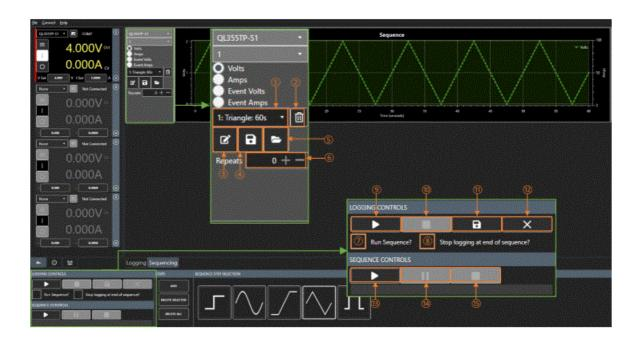
Steps that have been added to the sequence can be selected using the drop-down box ①. The steps are highlighted in the sequence with a background the same colour as the unit/event.
