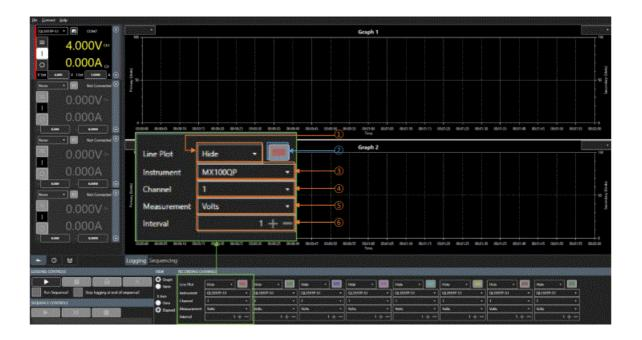
• Line Plot: Select the preferred graph ① to show the logged data on using the drop-down box. This can also be set to hide. The colour of the logging line can be selected from the colour picker ②.
