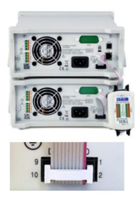
The Link Adaptor mates with standard 10W (2 x 5 DIL) female 2.54mm pitch IDC ribbon cable. Ensure the cable is fitted with the red stripe towards the black dot on the Link Adaptor and Pin 1 on the SMU. Strain relief has been added to the SMU connection end of the ribbon cable to protect the cable from potential damage when removing.
