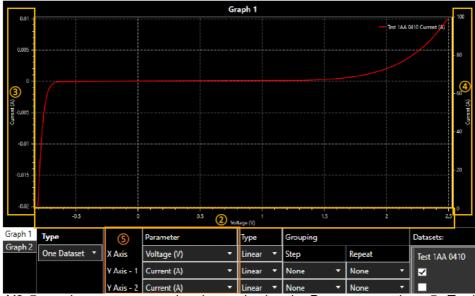
The X ②, Y1 ③ & Y2 ④ graph axes types can be changed using the Parameter settings ⑤. To show alternative parameter types from the loaded data, select an option from the drop-down box. The options are Voltage, Current, Power or Resistance, the X axis also include the options of Elapsed Time and Absolute Time.
