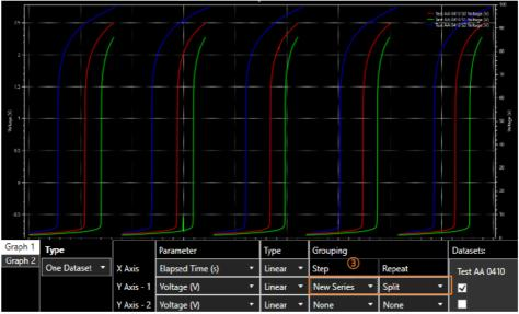
3. New Series / Split- Each step within the dataset is shown as a new series on the X Axis. Each repeat within the dataset is split within the series.
