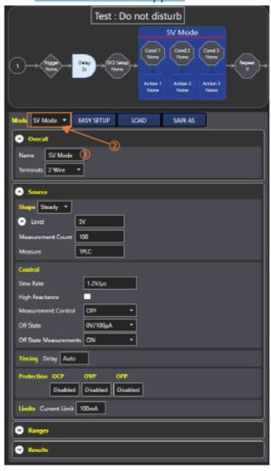
Selecting the mode box @ will show the mode editor @. It is possible to set the name of the mode and the step using Overall > Name @.
