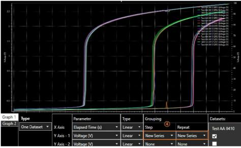
4. New Series / New Series- Each step and repeat within the dataset is shown as a new series on the X Axis.
