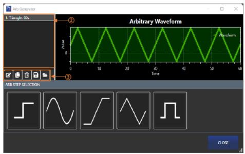
Steps are listed on the left-hand side ②, these can be selected and the following actions can be applied using the tools ③:
