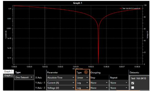
Each graph axis type can be displayed in either a Linear or Log (logarithmic) format using the Type settings ©.
