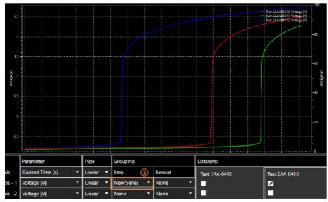
3. New Series – Each step within the dataset is shown as a new series on the X Axis.
