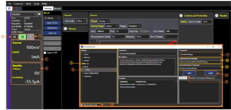
To run the setup, use the Run and Stop ① buttons. If the instrument is in a mode that uses the source, the source level and limit are shown in ②. The live primary and secondary results are shown in ③ unless the output is off, and off measurements are disabled.
