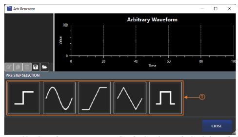
The Arb generator provides the tools to create a custom list of points that can be loaded as a list into a setup. A range of built-in step options are available, including: sine wave, square wave, triangle wave, ramp, and step. To add a step to the arb, select a shape from the options in the step selection ①.
