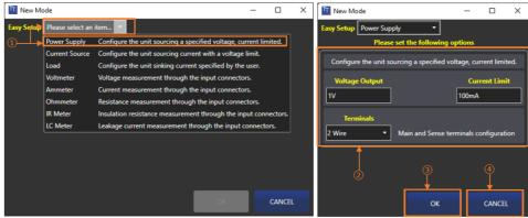
The Easy Setup menu contains a number of pre-configured setups, providing instant configuration for basic operational use of the SMU. Select the setup from the dropdown list ①. A brief description of the selected mode and mode specific options will become available ②, if no options are available only the description will appear. Enter the required values and select OK ③ to activate the mode with the set options, selecting Cancel ④ will close the window and no changes will be applied.
