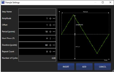
Each shape has a unique pop-up window that gives the editable parameters for that shape: Each step has the option to Insert, Add or Cancel:
