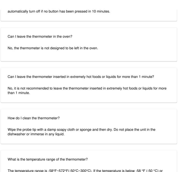
The temperature range is -58°F~572°F(-50°C~300°C). If the temperature is below -58 °F (-50 °C) or above 572 °F (300 °C), LL.L or HH.H will show on the display.
