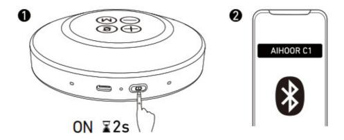
\*To disconnect and reenter pairing mode, double press the power button. To switch between Bluetooth and wired connection, press and hold the multi-function button for 2 seconds.
