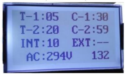
Calibration operation: press and hold the encoder to power the module to enter the calibration interface, the first flicker can be adjusted by the encoder once, after the third bit, the short press encoder can enter the operation interface. For example, the measured voltage is 220 V, the calibration interface can be set to 220.
