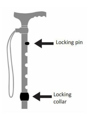
**WARNING** Prior to use always ensure that the locking pin fully protrudes from the selected hole position and by applying downward pressure on the handle of the walking stick has been assembled correctly.
