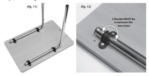
7. Insert the free ends of L shaped tubes into the H Frame (see fig. 13). You may require assistance to align them correctly. Slowly lower the table top (see fig. 13). Ensure you lower both sides at the same time to
