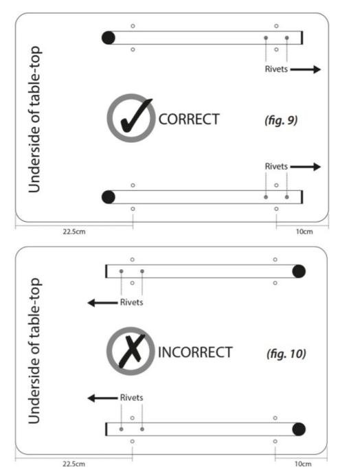
6. Attach the L shaped tubes using four C-shaped brackets and eight screws. (see fig.11) Ensure that the two C-shaped brackets nearer the edge of table are between the two rivets (see fig. 12). Do not overtighten as this may cause damage to the table.
