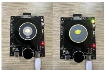
Finally, press the control end of the air conditioner to enter the control interface of the air conditioner, rotate the knob to select the degree of the air conditioner, press short to turn on the light of the air conditioner, and press long to exit the current interface.
