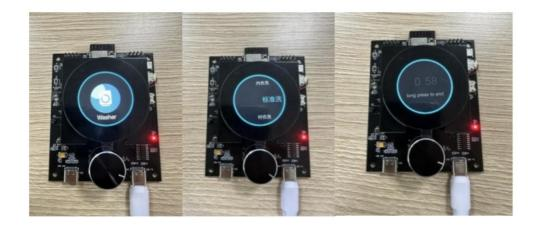
The second is the TV control end, short press to enter the TV station selection interface, rotate the knob and short press to select the station, at this time the remote control interface is displayed, there are various buttons, you can rotate and short press the knob to select, key buttons include volume adjustment, channel adjustment, etc. Hold down to exit the current screen.
