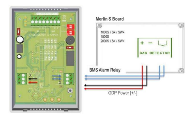
A relay will change state when in alarm or when gas is detected. BMS terminals can be used in conjunction with other external relays that affect other devices and controls such as purge fans and audible alarms etc.
