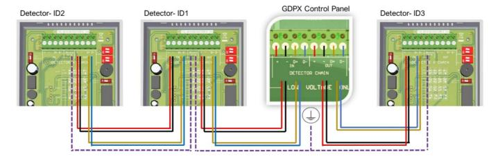
Reversing the [D+] and [D-] connections of any device can lead to the whole system stopping working owing to reverse polarity found on the terminals. In order to avoid this problem, it is recommended that a cable of same colour should be used to connect all [D+] terminals together and similarly cable of the same colour to be used to connect all [D-] terminals together.
