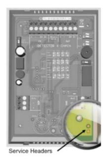
Access to the interior of the detector, when carrying out any work, must be conducted by a competent person! It is recommended to bump test detector(s) prior to resetting the service reminder message!
