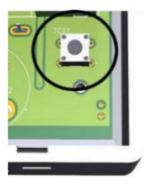
When the test button on the circuit board is pressed and held the detector will simulate an open circuit to ensure configured systems, outputs, alarms, indications, and other external devices operate as intended in response to gas. When the test button is released – the test sequence will terminate and return to normal operation.
