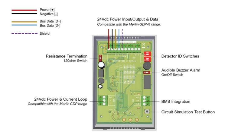
Be careful when creating access for cables – Damage to circuit boards will void any warranty! Any damage attempting to remove the circuit board parts may void any warranty! Detectors must be earthed/grounded for electrical safety and to limit the effects of EMC or R/F interference! For MODBUS communications, a shielded cable is used!
