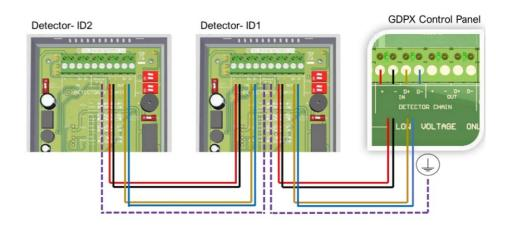
**Split Detector Chain from Control Panel example**
