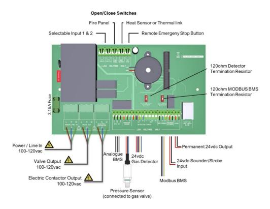
**Note:** Terminal blocks are plug/socket type and may be removed to ease wiring.
