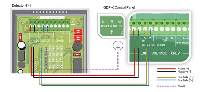
[SHEILD WIRE] detector terminals are used for earthing/grounding and shield wires connected to any earth/ground terminal on the control panel. Twist the shield wire to avoid stray shield wires. If the detector does not have dedicated shield wire terminals, shield wires connect to the 24vdc negative terminal [-] on both detector and panel.
