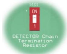
If a split chain is used, terminate the last detector in each chain.
