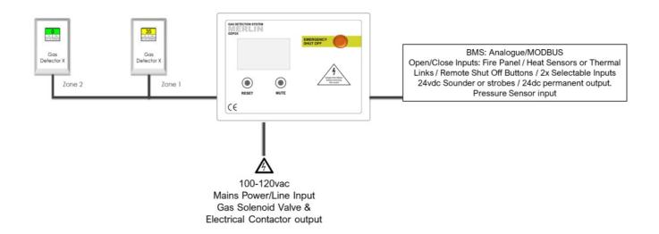
Where detector cable runs may exceed 100 yards from one control panel – Contact your supplier! The use of sound strobes are highly recommended!
