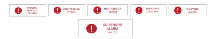
Alarm messages from terminals [INPUT 1] or [INPUT 2] will depend on the name selected in the settings. For example, if CO is the selected input the alarm message will display "CO sensor alarm". If [FAN] is the selected input, you will see "fan fault". All alarm screens will show the input terminal used i.e. Input 1 or Input 2.
