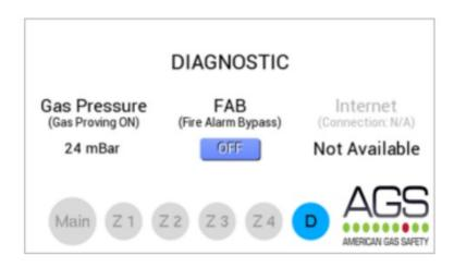
Fire Alarm Bypass (FAB) This is an enable/disable feature where fire alarm tests may be required. To enable the FAB feature select the press the off/on button shown where prompted to confirm the action prior to activation. The FAB feature is displayed on screen when enabled. The system will return to normal at the end of the pre-selected time of 15, 30 or 45 minutes configured in the settings. You can manually disable the FAB by pressing the blue option box to OFF on the diagnostic screen.
