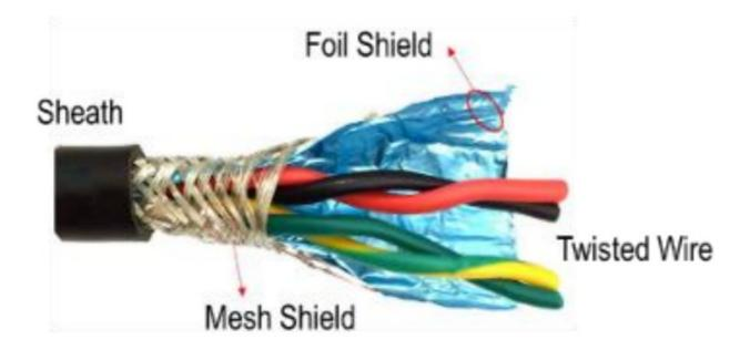
A shielded and twisted 2 or 4 core cable is used to wire the MODBUS terminals [D+ & D-). The shielding can be of 2 types: braided [mesh of thin conducting wires] or foil (consisting of a thin sheet of metal covering the twisted wires). One example of such cable is BELDEN 3082A. Any cable with similar characteristics can be used to connect all the devices together.
