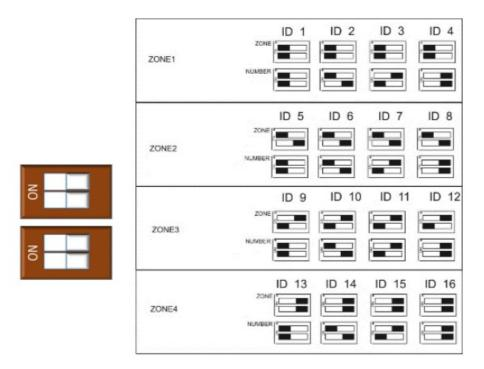
The ID configuration diagram is printed onto detector boards for quick reference as shown opposite. All detectors are factory set to ID1.
