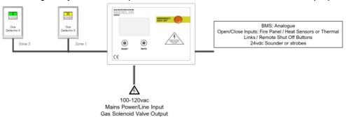
Where detector cable runs may exceed 100 yards from one control panel – Contact your supplier! The use of sound strobes are highly recommended! Refer to your detector manual for further information regarding coverage, location and positioning including areas and conditions to avoid!
