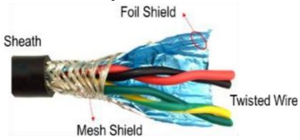
If you are encountering noise or irregular problems with a bus link, the problem is likely related to grounding, incorrect shielding or wiring mains power cables next to data cables.
