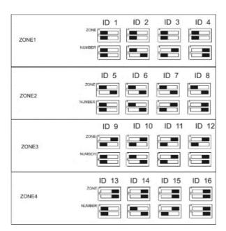
We recommend a plan, map and/or marking the detector enclosures detailing ID and location! ID Switches must be configured for each detector connected to receive and display accurate data!
