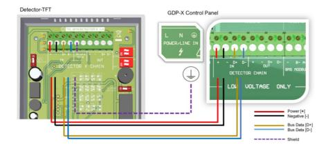
**[SHEILD WIRE]** detector terminals used for earthing/grounding and shield wires connected to any earth/ground terminal on the control panel. Twist the shield wire to avoid stray shield wires. If the detector does not have dedicated shield wire terminals, shield wires connect to the 24vdc negative terminal [-] on both detector and panel.
