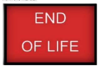
At the end of its predicted operational life – the detector will display an 'End of Life' screen. This message indicates that the detector has reached its expected operational lifecycle and no gas levels are displayed. You must contact your supplier immediately for replacement.
