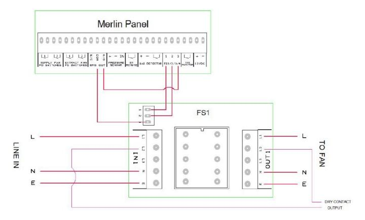
BMS Selection DIP switch on Merlin utility panel has to be set to ON position!
