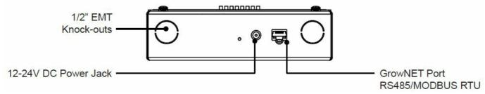
**Maximum 1A power supply current! An input** power protection fuse of 1A is required to prevent damage to the unit from overloading.
