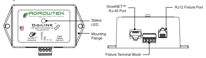
Fixtures connect to either the RJ-12 connection (see compatible fixtures above) or via manual connection to the terminal block. See wiring diagrams for connection details. A status LED will flash when communicating with the GCX controller.
