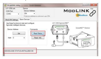
6. Set the device address to the desired value by selecting the "Addr." drop down then press "Set."
