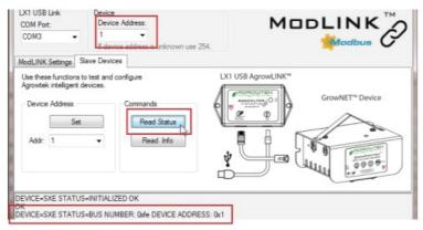
8. The device is ready to be deployed on a MODBUS network. Set the Device Address in the Connection box back to "254" to connect to the next device.
