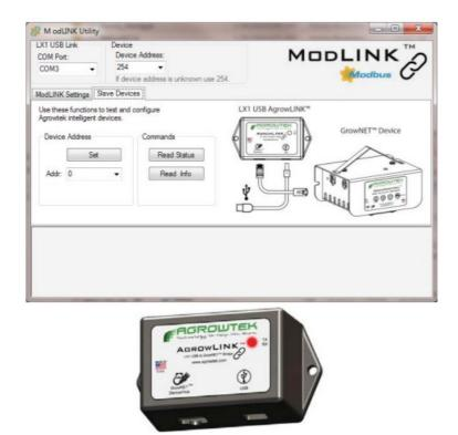
The LX1 USB AgrowLINK may be used to confi gure the LX2 ModLINK and set device (slave) addresss of devices.
