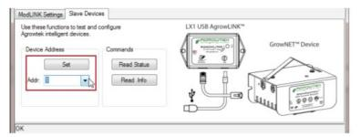
7. Verify the new address by selecting the new address in the Connection box then press "Read Status."
